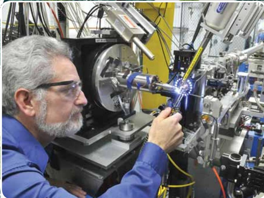
Robert Fischetti, a beamline director at the Advanced Photon Source, a national synchrotron X-ray research facility at the Argonne National Laboratory, adjusts a sample crystal on a beamline. *Photo courtesy of the Argonne National Laboratory.*
